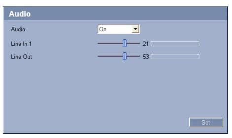
You can set the gain of the audio signals to suit your specific requirements. The current video image is shown in the small window next to the slide controls to help you check the audio source and improve assignments. Your changes are effective immediately.
